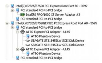
Windows Device Manager with 2 PCIe to PCI Expansion Systems Installed in a "Fan-Out Configuration.
